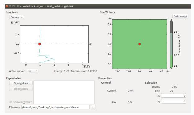
Note that the transmission peak has shifted down in energy as compared to the non-twisted ribbon. The twist represents a source of electron scattering, since it breaks the translational symmetry of the non-twisted ribbon electrodes along the transport direction.
