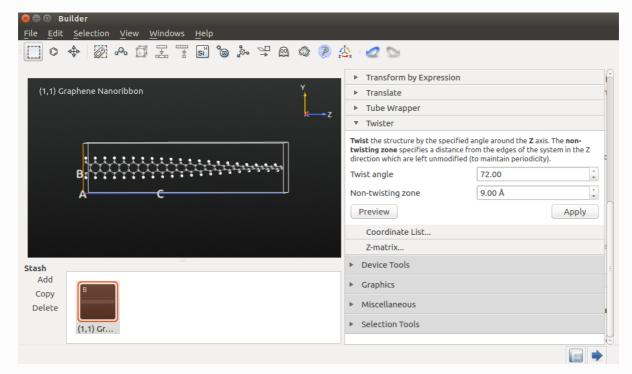
Certain parts of the system to the left and right of the structure are not twisted; the length of the non-twisted part is specified by the value of "Non-twisting zone". The rest of the structure is twisted by the
