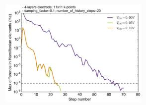
• If slightly less aggressive mixing parameters are used compared to the default ones (lower damping\_factor and number\_of\_history\_steps), the convergence at zero (finite) bias voltage is slightly slower (faster).
