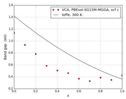
We see that the band gaps show a qualitatively correct trend, but with rather large deviations in the Ga-rich region on the left and a bit of an oscillation on the right. Fortunately, it is possible to fit the c-parameter of TB09-MGGA to reproduce the correct band gaps of the end-points, which should also improve the band gaps in the intermediate region.
