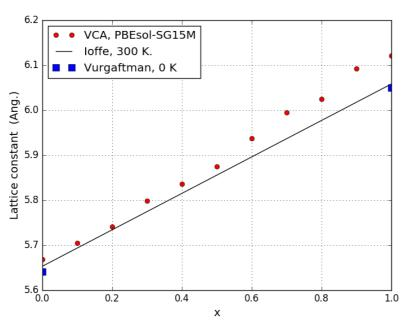
We see that the experimental lattice constants are well reproduced in the Ga-rich region on the left of the figure, while the deviation is higher, about 1 %, in the In-rich region on the right. This is in line with general expectations, as PBEsol is designed to give accurate lattice constants, while GGA-type functionals generally overestimate them.
