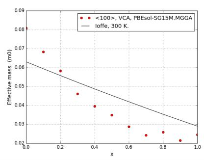
We see that the effective mass of GaAs is overestimated, leading to an overall distortion of the shape of the curve. However, it does capture the overall downwards trend in the effective mass from GaAs to InAs.
