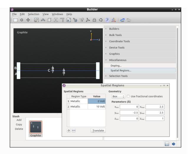
The applied voltage results in 4 V/nm in the z direction, just above the field that has been found in experiments to open a band gap.
