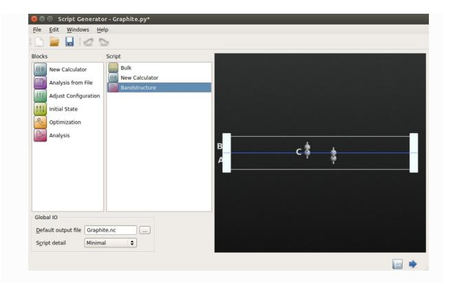
8. Double-click the **Bandstructure** block and change the route to G, M, K, G. Also increase the number of points per segment to 200.
