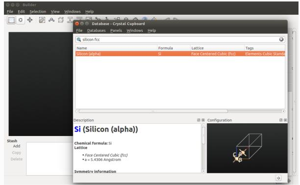
In the Builder, use the Builders ➤ Surface (Cleave) tool to create the Si(100) facet:
