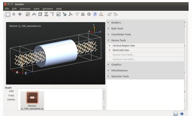
Then send the device configuration to the **Script Generator**.
