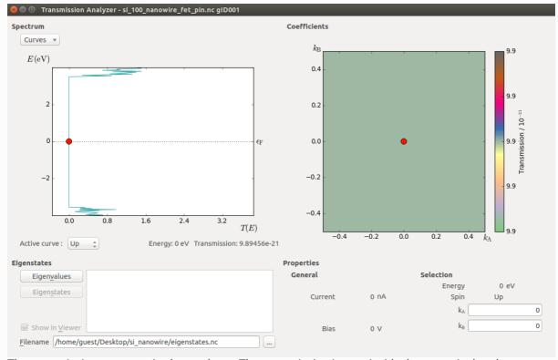
The transmission spectrum is shown above. The transmission is zero inside the nanowire band gap, which appears to be roughly 7 eV, significantly larger than computed earlier. This is due to the p- and n-doping, which has moved the valence and conduction band edges with respect to the Fermi level.
