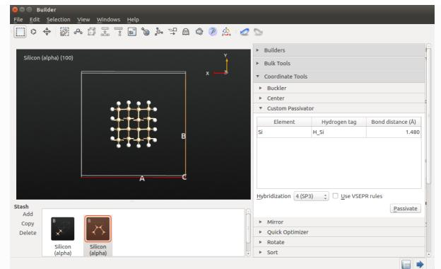
Send the H-passivated Si(100) nanowire to the Script Generator by using the in the lower right-hand corner of the Builder window.
